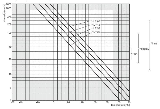
The correlation between viscosity and temperature usually is described in the double logarithmic diagram above.
