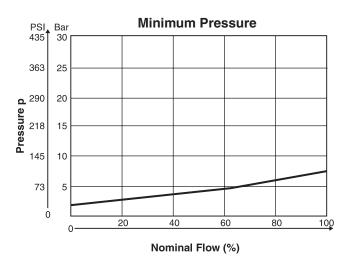
The performance curves are measured with external drain. For internal drain the tank pressure has to be added to curve.
